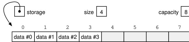
Fig. 4. Used area on the left and supply area on the right. Same indexing in the native array and in the user interface.
